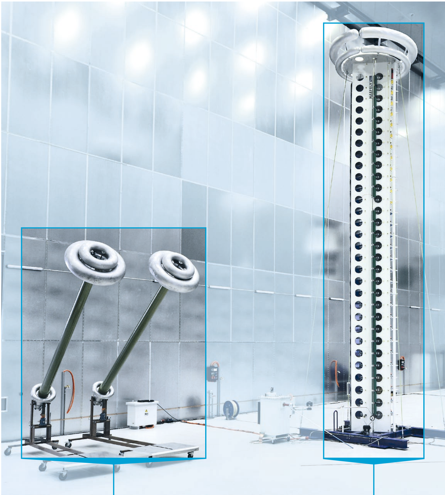
Water-insulated cable termination system CTT 800 AC voltage: 800 kV Lightning impulse voltage: 1900 kV Switching impulse voltage: 1200 kV Dimensions: 5.2 × 1.9 × 1.5 m
